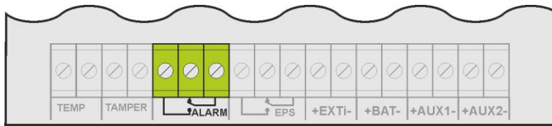
Fig. 9. Technical output ALARM.
